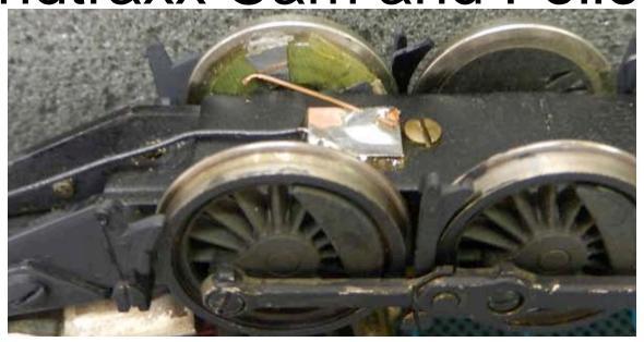
If you get a double chuff from a lobe, turn the completed model over in a foam cradle and attach some alligator clips from the track leads, one to the loco and one to the tender. Run the loco slowly to find the lobe causing the double chuff. Usually light sanding with 600 grit stick or changing the bend in the follower will eliminate the double chuff.
