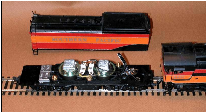
Two oval speakers were installed in the floor of the Daylight tender. The Tsunami decoder was install in the engine.
